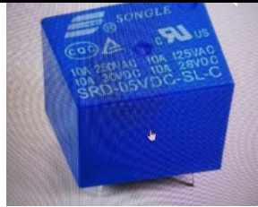
Figure-5- spdt relay
